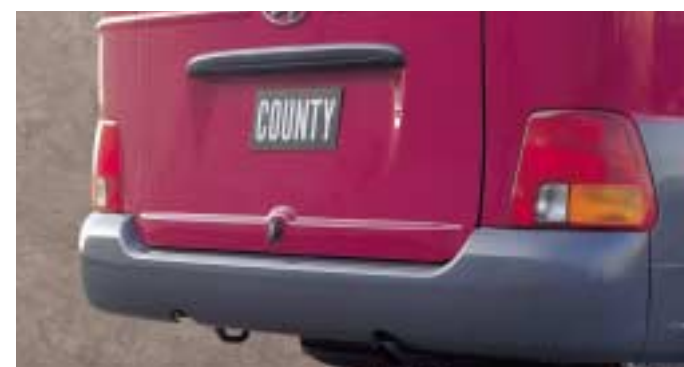
Rear Bumper One piece-type steel bumper is gently rounded around the edges for a soft look that matches the overall design theme.
